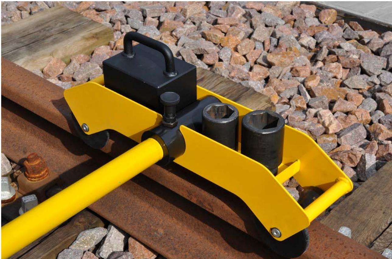
Picture 1: Cross arm and balancing carriage
