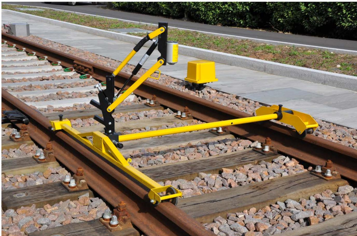
Cembre presents CS-EU, the new support trolley designed for railways application. The new trolley allows to carry and use all Cembre impact wrench or sleeper drilling machines. The restyling of renowned Cembre CS-SD support trolley includes now some special kit to be more convenience than previous version increasing the versatility in application.
