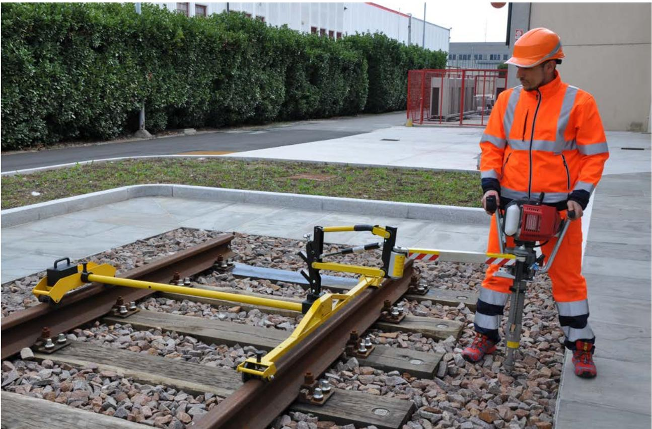
Picture 4: CS-EU with KLE extension and balance cross arm with proper counterweight
